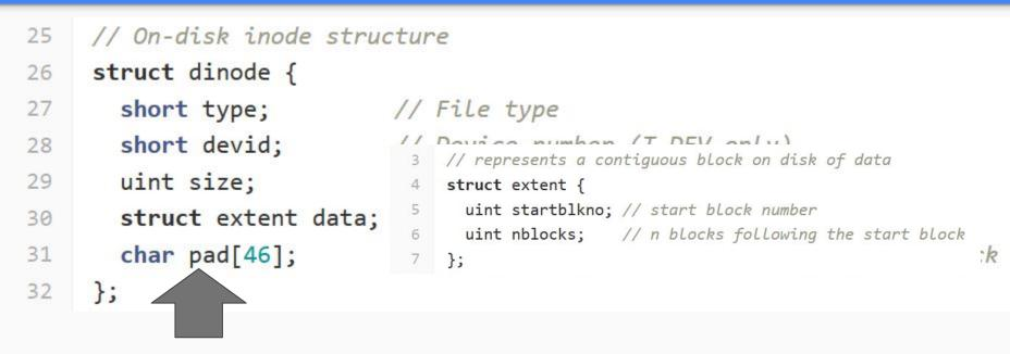
Padding ensures there is always a whole number of dinodes on a block (i.e. BLOCK\_SIZE % sizeof(dinode) == 0, so no dinode is split between blocks)
